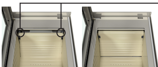
Remove the fuse, then remove the smoke deflector plate by pulling forwards and downwards
